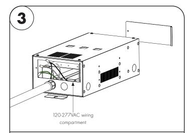
**3.1** Connect the white (neutral) and black (hot) power supply wires to the white and black power wires (120 - 277 VAC). Followed by connecting the ground wires in accordance with local electrical codes.
