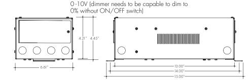
Surface mounted with conduit access
