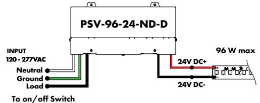
**Enlighted Enabled Dimming Power Supplies 120VAC - 277VAC**
