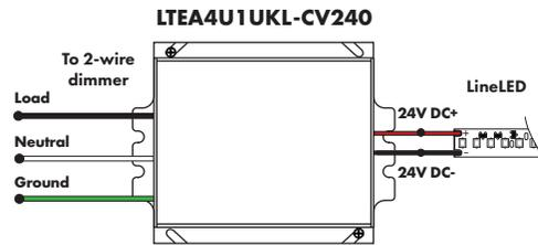
**DMX Dimming Power Supplies 120VAC - 277VAC**
