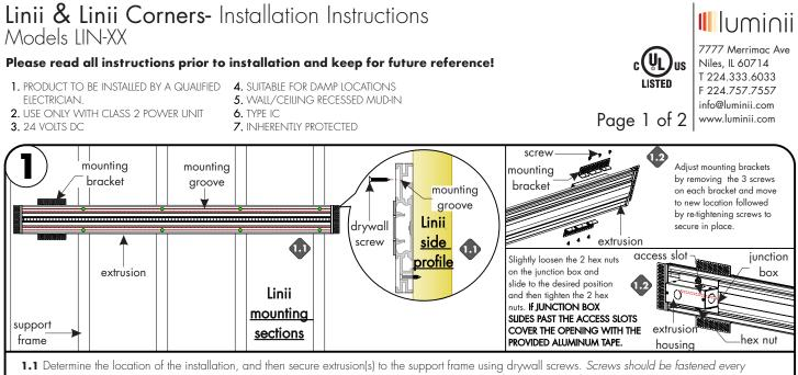
16-18" depending on support frame and also at the ends of extrusion. Follow diagram above for additional information. Make sure screw is fastened through mounting grooves on the extrusion housing. Mounting brackets should be used when support frame not available. (reference step 4 for more details).
