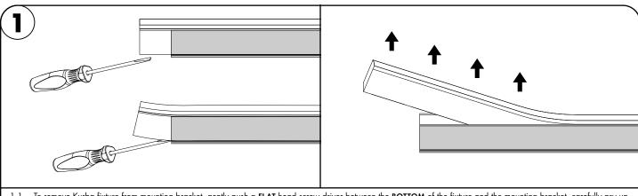
To remove Kurba fixture from mounting bracket, gently push a FLAT head screw driver between the BOTTOM of the fixture and the mounting bracket, carefully pry up the Kurba Fixtrure. Once Kurba fixture has started coming out of the bracket, stop using the screw driver and instead use your hands and fingers to pull the fixture out of the bracket making sure to keep it at a 15° angle.
