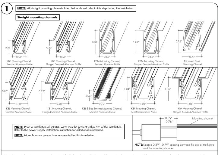
Once the location or pattern is determined for Kurba to be installed, start off by marking the area. Amount of brackets may vary dependant upon pattern. Reference diagrams below.
