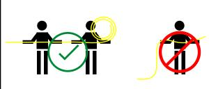
When light length longer than 6ft, make sure somebody helps to lift the light, in case the heavy weight of light itself generates too small bending angle or twisting, which may damage Kurba.
