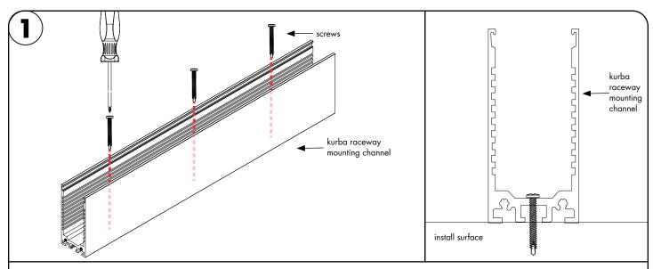
1.1 Mark the desinated space prior to install. Drill holes into the surface, followed by placing the mounting channel to the surface. Make sure its straight by using a level. Use screw to secure the channel.
