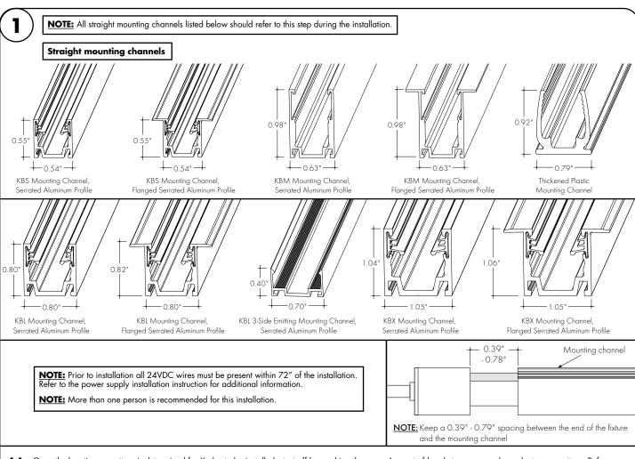
Once the location or pattern is determined for Kurba to be installed, start off by marking the area. Amount of brackets may vary dependant upon pattern. Reference diagrams below.
