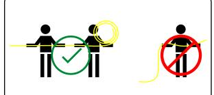
When light length longer than 6ft, make sure somebody helps to lift the light, in case the heavy weight of light itself generates too small bending angle or twisting, which may damage Kurba.
