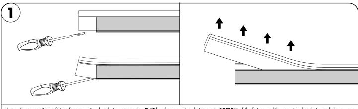
1.1 To remove Kurba fixture from mounting bracket, gently push a FLAT head screw driver between the BOTTOM of the fixture and the mounting bracket, carefully pry up the Kurba Fixtrure. Once Kurba fixture has started coming out of the bracket, stop using the screw driver and instead use your hands and fingers to pull the fixture out of the bracket making sure to keep it at a 15° angle.
