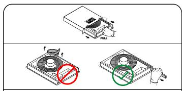
When unpacking Kurba, carefully pull it out of the packaging box. Note: Incorrect unpacking may cause PCB fracture or damage on electronic components, and lead to the failure of light. Gloves are recommended in third step
