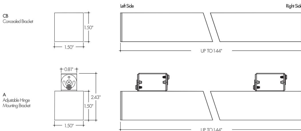
Adjustable Hinge Mounting Bracket is not available on system runs with corners
