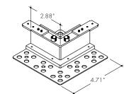
For creating a 90° in-plane corner. For use with FF Front Flange and ST-JOIN-E-F Electrical Joiner only.
