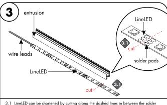
3.1 LineLED can be shortened by cutting along the dashed lines in between the solder pads. Make sure the cut is made on the side of the LineLED without the wire leads. LineLED cannot touch the metal endcap which will shorten the circuit.
