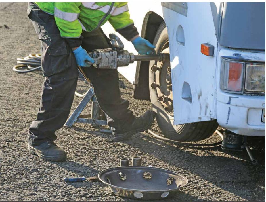
and have those corrected Be specially aware of high heat on tires, which may be immediately. If you chose not to replace the tire, it should be caused by ambient and road dismounted and plugged from temperatures, under-inflation the inside rather than the outor excessively pumping the side for best performance. Do brakes. Invest in a tire-monitora follow-up pressure check ing system that will alert you to
