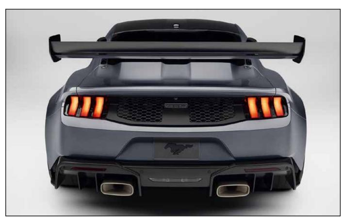
A hydraulic system can change the angle of the giant rear wing on the Mustang GTD, helping it go faster in straight lines and create more downforce in corners.
