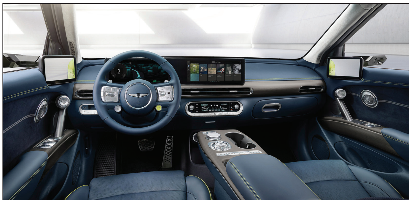
The GV60 can be started without a key using biometric scans. A facial recognition camera on the door and fingerprint scanner on the center console can identify the owner.
